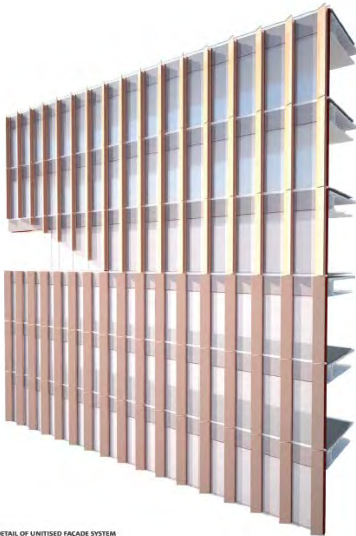
DETAIL OF UNITISED FAÇADE SYSTEM
